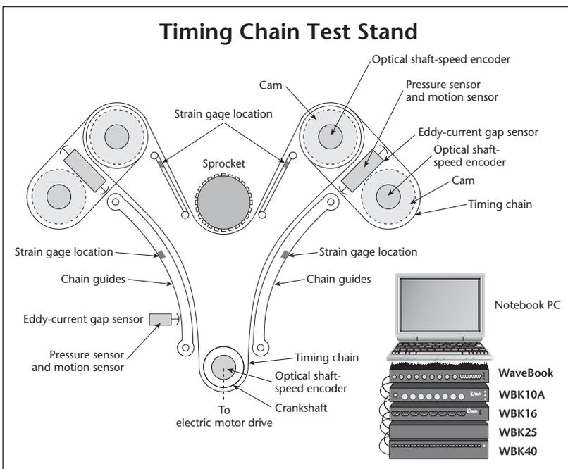
Several test stands in U.S. Tsubaki's test laboratory are instrumented and outfitted with chains, sprockets, tensioners, cams, and guides to simulate a number of different engine configurations. An electric motor drives the system to run product validation and life tests while an IOtech WaveBook records the data. The test stands are particularly useful when an engine is not yet available to be fitted with a timing chain system.
