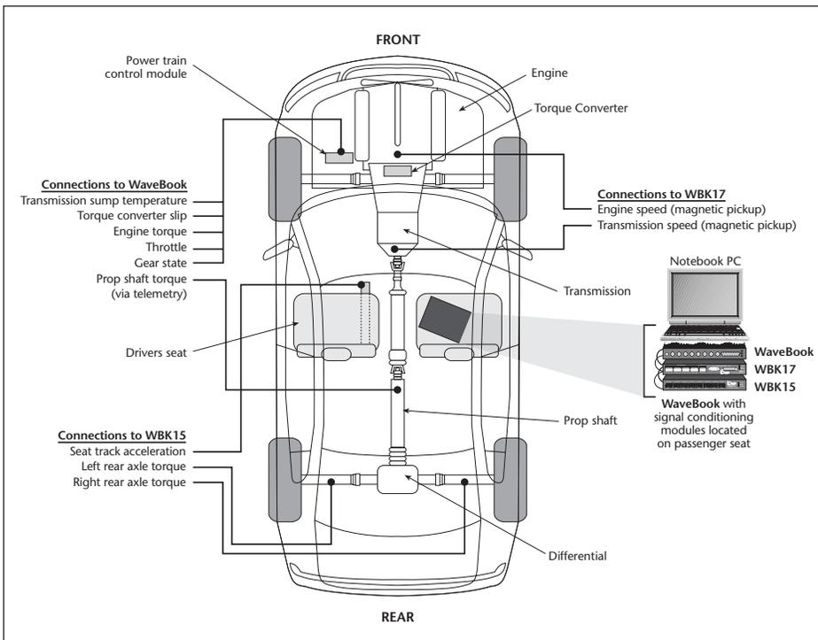
The Powertrain Div. of General Motors records and analyzes test data collected from torque converters during on-vehicle tests and engine test stands. Engineers use the data to characterize high-performance cars and fuel-efficient commuters to achieve optimum durability and drivability. The WaveBook's portability, compact size, and intuitive interface allow the engineers to change easily from instrumenting a vehicle to setting up a test stand or changing acquisition structure.
