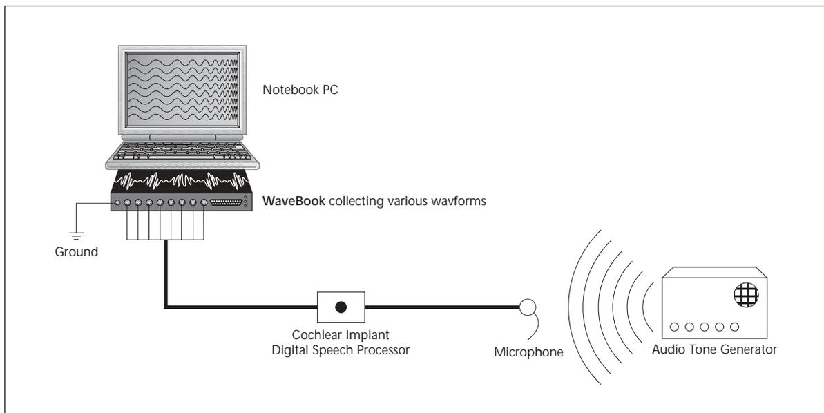
Connected to a notebook PC, the WaveBook processes a variety of waveforms. This data is used to program special software for fine-tuning cochlear implants — enabling the profoundly deaf to hear.
