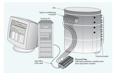
Variations in temperature distribution within the kiln are measured with several thermocouples strategically located to establish which of several heaters need to be adjusted for higher output. The thermocouples feed individual signal conditioner modules, which in turn connect to the Personal Daq for processing. The computer and Personal DaqView graphical data acquisition and display software provide permanent records and a hard-copy printout of the temperature profile for customers.
