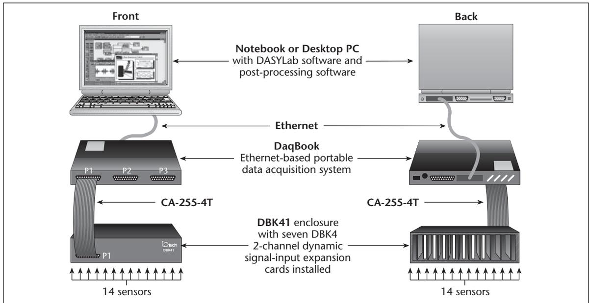
Garrett Smith at Ball Spin Engineering uses a variety of sensors for measuring relatively large vibrations and displacements in heavy equipment such as hydroturbines and much smaller vibrations in semiconductor processing facilities. The IOtech **DBK4** signal conditioners, **DaqBook** data acquisition system, and **DASyLab** software let Smith measure these data in real time and record them for subsequent post processing.
