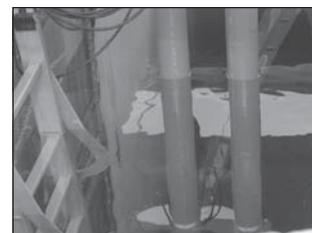
Shell's test lab includes a water tank where pipe collisions simulate the motion of an oil rig's support structure under hydrodynamic conditions. IOtech [DaqBooks](#) and [WaveBooks](#) collect the high-frequency vibration signals generated so engineers can analyze improved structural designs.
